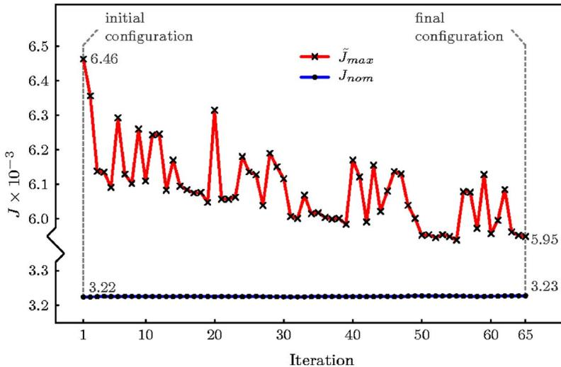
FIG. 5. (Color online) Performance of the robust local search algorithm. The worst case cost for the final configuration  $\mathbf{p}_{65}$  is improved by 8% compared to  $\mathbf{p}_1$ , while the nominal cost remained constant. The overall improvement of the robustness is 90%.
