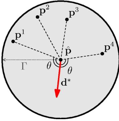
FIG. 4. (Color online) A two-dimensional illustration of the neighborhood  $\{\mathbf{p} \mid \|\mathbf{p} - \hat{\mathbf{p}}\|_2 \leq \Gamma\}$ . The solid arrow indicates an optimal direction  $\mathbf{d}^*$  which makes the largest possible angle with the vectors  $\mathbf{p}^i - \hat{\mathbf{p}}$  and points away from all bad neighbors  $\mathbf{p}^i$ .
